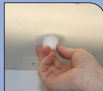
Simple oxygen sensor calibration without removing the sensor from the chamber
